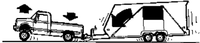
Top heavy loads can cause trailer "dive" under hard braking, possibly reducing steering and braking control.
